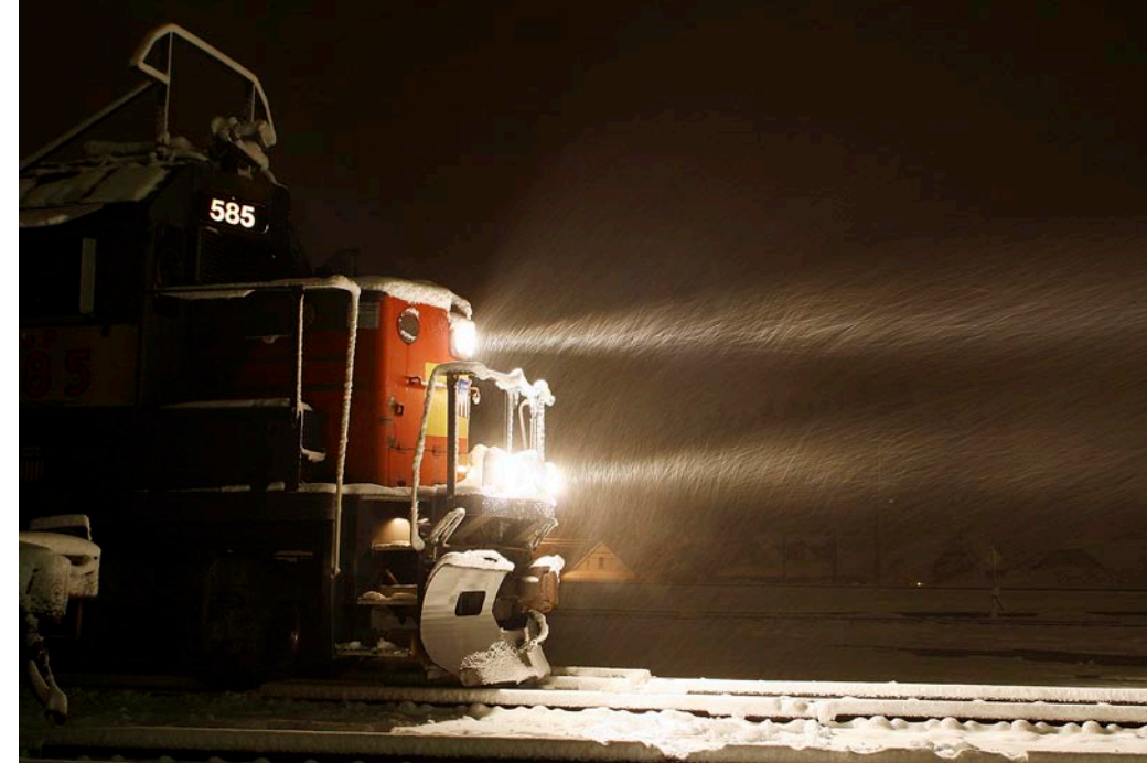
Blizzards dimming visibility: Union Pacific GP38-2 585, modified with a flanger for snow removal, waits to leave the maintenance-of-way yard in Truckee, Calif., on March 28, 2006. Ray Lewis
